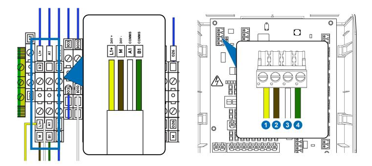
To connect the external communication box to the unit, connect terminal X2 on the main machine to terminal X1 on the communication box.
