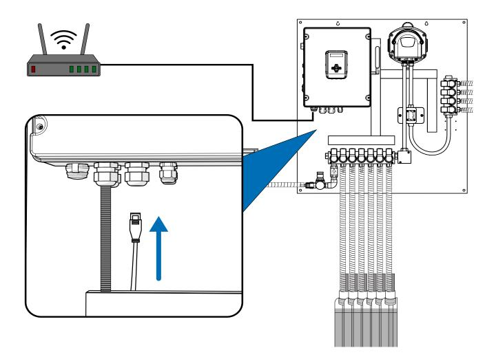
To connect your unit to the internet, simply plug an Ethernet cable into any router through the connector located on the bottom of the main box.
