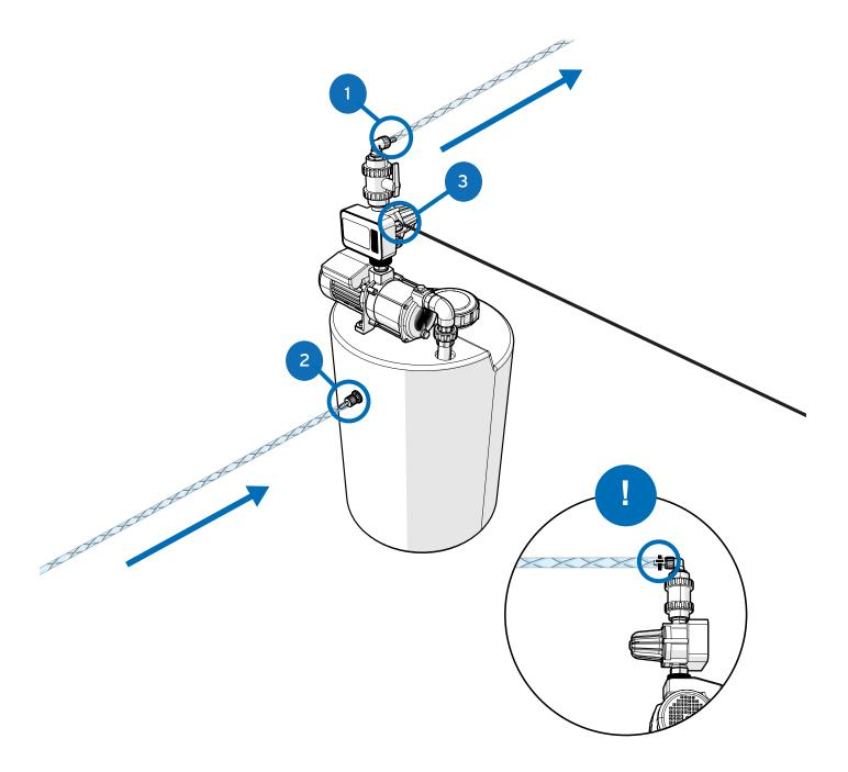
Please note that the unit requires a flow rate of min 2/l per min - max 10/l per min and a dynamic pressure range of 1.5 bar (min) - to 3 bar (max). A booster tank is recommended whenever a consistent supply is not available.
