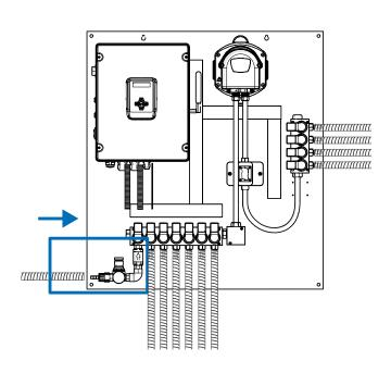
Connect the water supply to the water inlet connection seen on the unit here.
