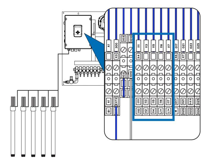
To connect the external suction lances to the machine, utilize inputs I10 to I17, as indicated above.
