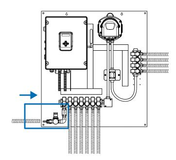
Connect the water supply to the water inlet connection seen on the unit here.
