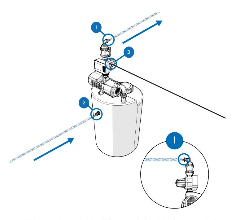
Please note that the unit requires a flow rate of min 68 fl oz/min - max 339 fl oz/min and a dynamic pressure range of 1.5 bar (min) - to 3 bar (max). A booster tank is recommended whenever a consistent supply is not available.
