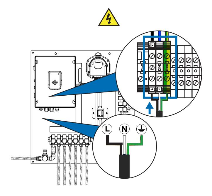
For the power supply of the equipment you must use 3x16 AWG cable. Insert the cable through the channel located at the bottom left and use one of the cable glands to insert it safely inside the control cabinet. Connect to the terminals identified with X1 found on the lower left of the connections.
